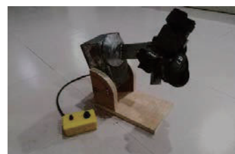
Fig 5 : The finished tracking Mount with Sony A7II camera attached.
